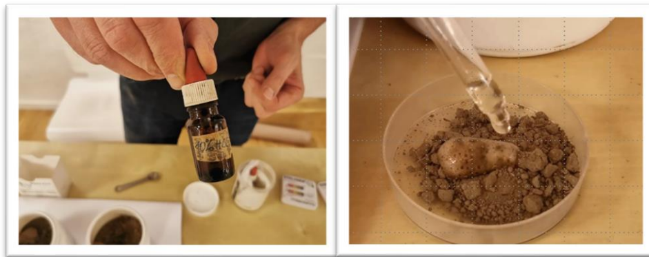
10% hydrochloric acid (left) and foaming reaction in the presence of carbonates (right)
