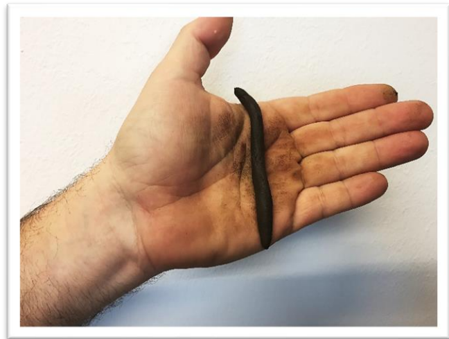
Austrian texture triangle according to ÖNORM L 1050 (left) and soil material rolled into ribbons (right)
