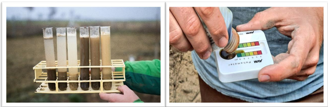
Determination of aggregate stability (left) and pH value in neutral salt (right)
