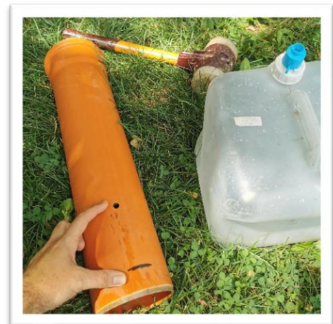
PVC pipe with marked depth and indicated filling height (10cm)
