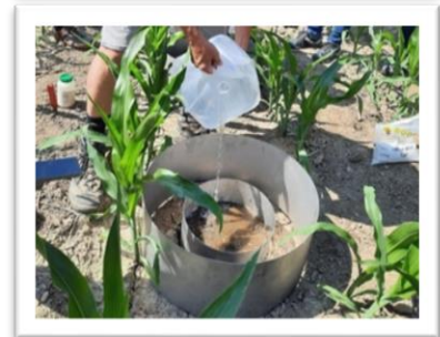
Measurement of infiltration with PVC pipe (above) or double ring infiltrometer (below)
